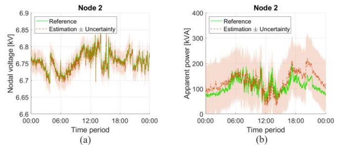
Figure 7: Time-series of the estimated voltage (a) and nodal apparent power flow (b) at the unmonitored node 2.
