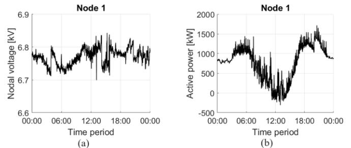
Figure 2: Time profiles for one day of voltage (a) and active power flows (b) at the primary substation.
