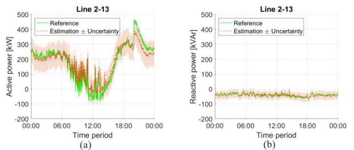
Figure 5: Time-series of the estimates active (a) and reactive (b) powers on the unmonitored line 2-13.
