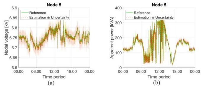
Figure 8: Time-series of the estimated voltage (a) and nodal apparent power flow (b) at the unmonitored node 5.
