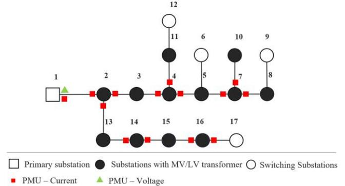
Figure 1: Single line diagram of the selected MV feeder.
