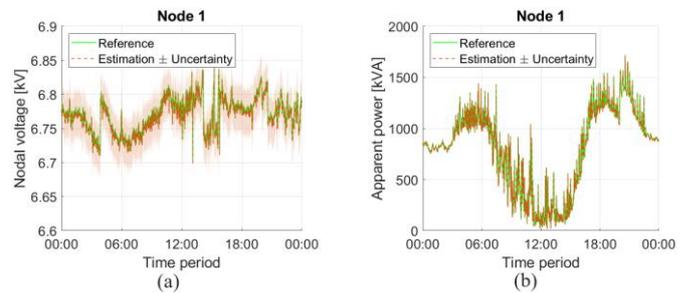
Figure 6: Time-series of the estimated voltage (a) and nodal apparent power flow (b) at the monitored node 1.
