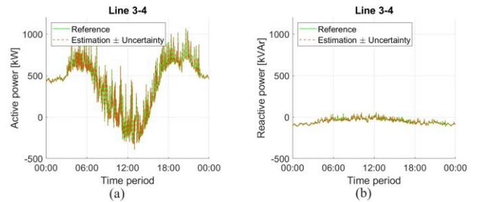
Figure 4: Time-series of the estimated active (a) and reactive (b) powers on the monitored line 3-4.
