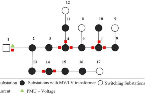
Figure 3: Single-line diagram illustrating the considered measurement configuration.
